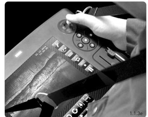
**B) Relative articulation** means scanning the application step by step. By moving the joystick, the probe head follows slowly in the desired direction. After you stop moving the joystick, the probe head remains in it's position. You can correct the position by directing the joystick to another position. To redirect the probe head into it's standard position (straight, not articulated), press the joystick. See pictures 1.1.3d to 1.1.4e or "Extended settings" on page 20.
