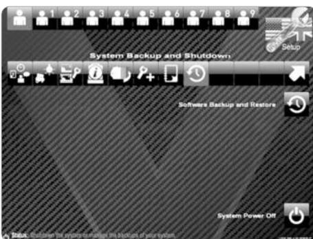
After pushing „System Power Off”, please wait for the shutdown screen to occur and turn off your system with the main switch.
